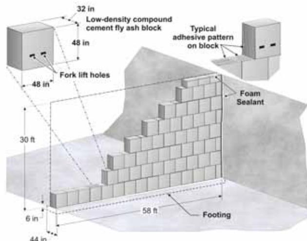
Figure 1.—Schematic of the Super Stopping for use in large-opening mines.
