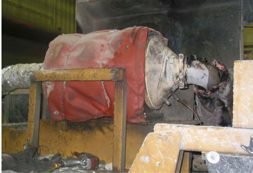
Figure 1.—Engelhard DPX DPF system on truck #92128.
