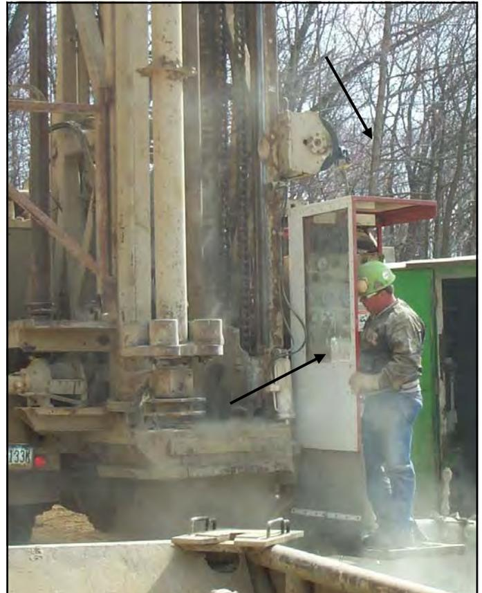
NIOSH has developed a partial cab design (arrows note cab on rig) that can be retrofitted onto drilling rigs. Field tests have shown that the partial cab can reduce sound levels at the operator's ear by as much as 8 dB(A) while hammer drilling.
