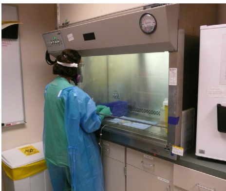
Figure 1. Veterinary technician wearing PPE while preparing chemotherapy drugs in a Class 2 BSC.
