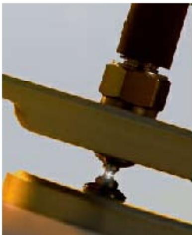
When the sample apparatus is closed, the sample arm slightly compresses the droplet and a sample column is drawn. Surface tension alone holds the sample in place. The spectral measurement is then made and quantification is made based on the tightly controlled path length of 1 mm.
