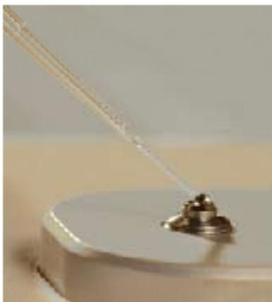
With the sample apparatus open, a droplet of sample is pipetted onto the measurement pedestal.
