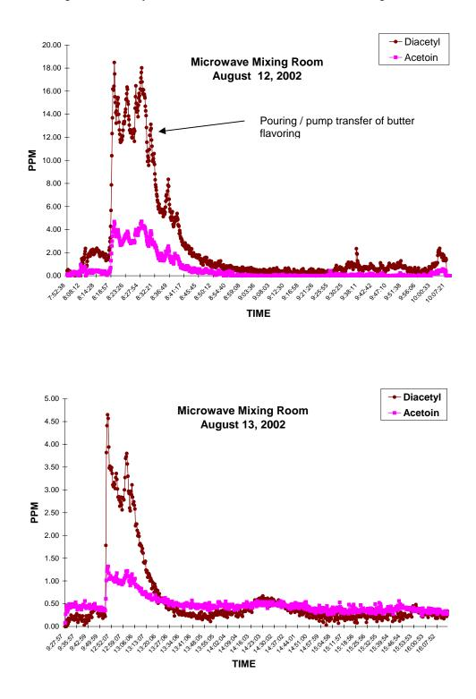
Figure 3. Diacetyl and acetoin air concentrations in the mixing room.
