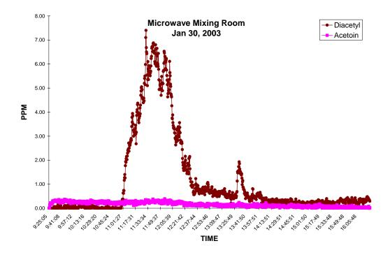
Note: The peak exposures for diacetyl and acetoin are from butter flavor handling / mixing operations.
