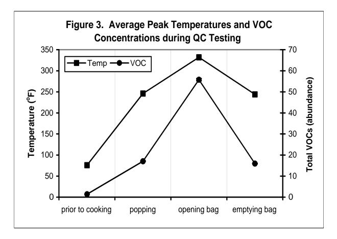
\*Figure 3 Legend: Measurements of peak temperature and VOCs during four steps in the QC process. Each point presents the average of readings taken during QC testing of ten different bags of popcorn.
