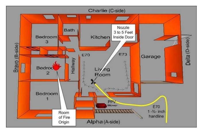
Figure 2. Location of E70 nozzle, positive pressure ventilation, and search patterns of E70 and E73.
