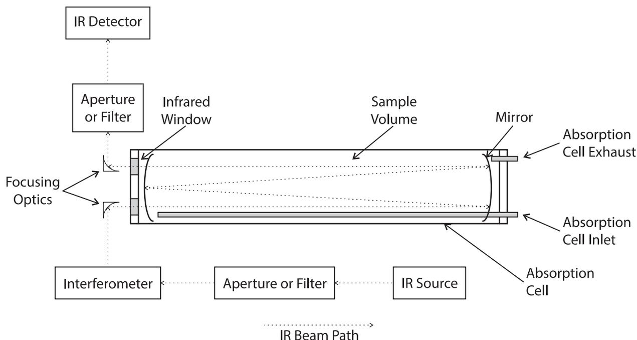
**Figure C1. FTIR spectrometer components and beam path.**
