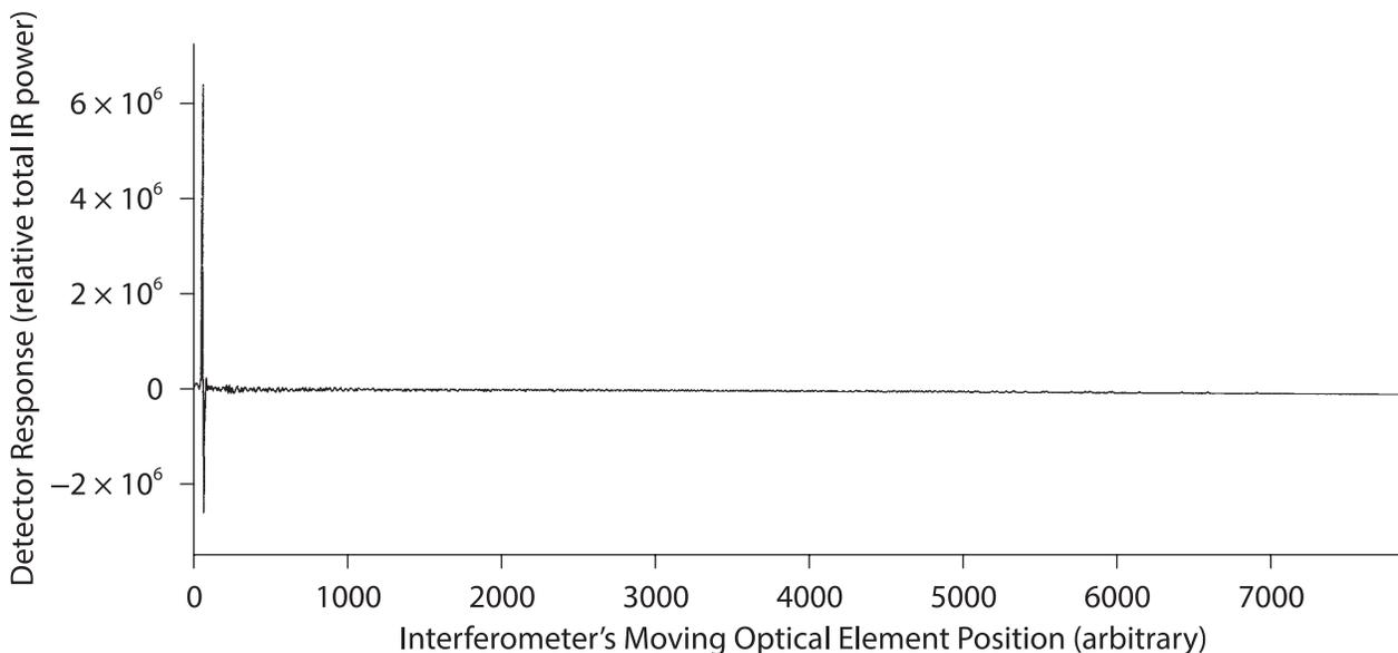
Figure C3. Mid-infrared interferogram.
