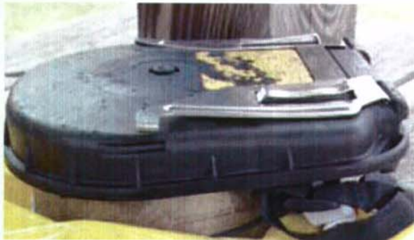
Figure 9. Dented Draeger OXY K-Plus Belt-Clip
