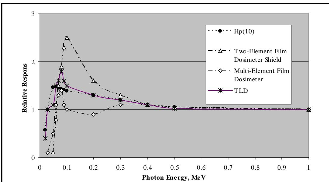
Figure A-2. Measured deep dose response for Hanford two-element film, multielement film, and thermoluminescent dosimeter compared to  $H_p(10)$  (Wilson et al. 1990).
