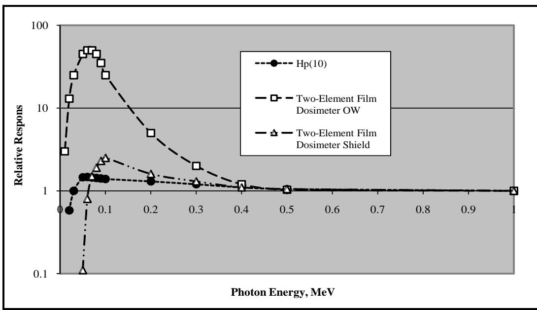
Figure A-1. Measured two-element dosimeter photon response for AP exposure geometry (Pardue, Goldstein, and Wollan 1944; Wilson et al. 1990).
