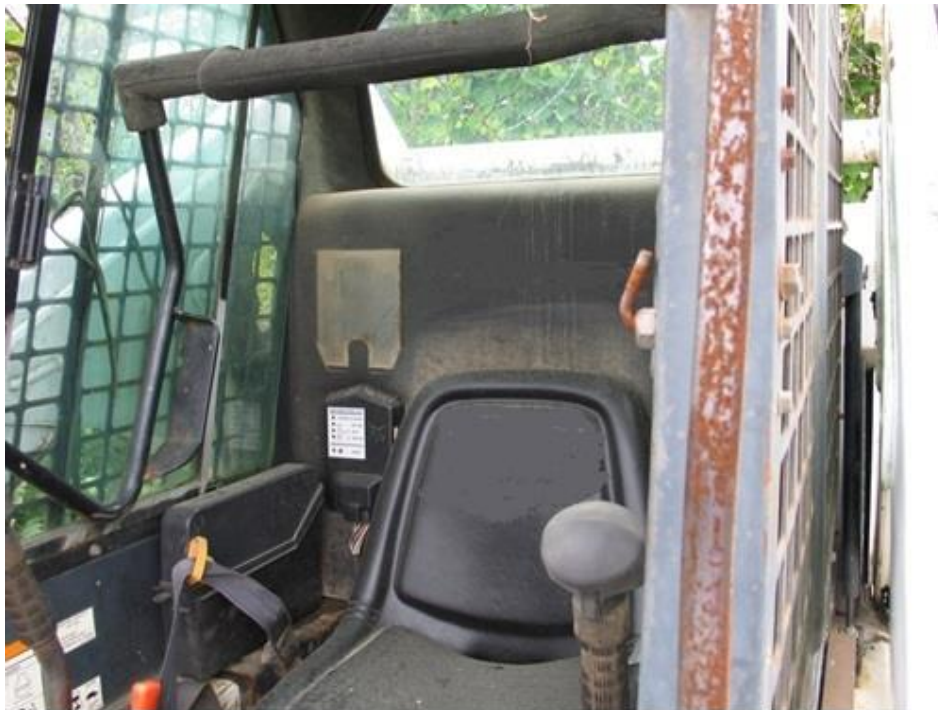
Figure 4 – Skid-steer loader's seat bar and lever controls
