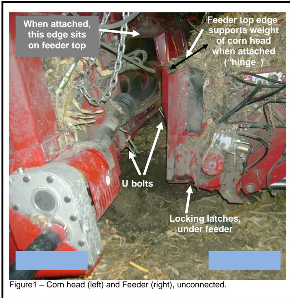
Figure1 – Corn head (left) and Feeder (right), unconnected.
