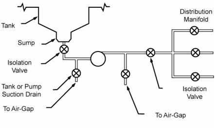
Figure 8 - Potable Storage Tanks Drains
