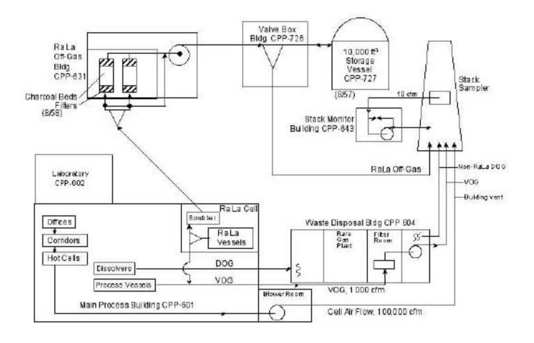
Figure 2-11 RaLa and Idaho Chemical Processing Plant off-gas flow schematic, 1957–1959
