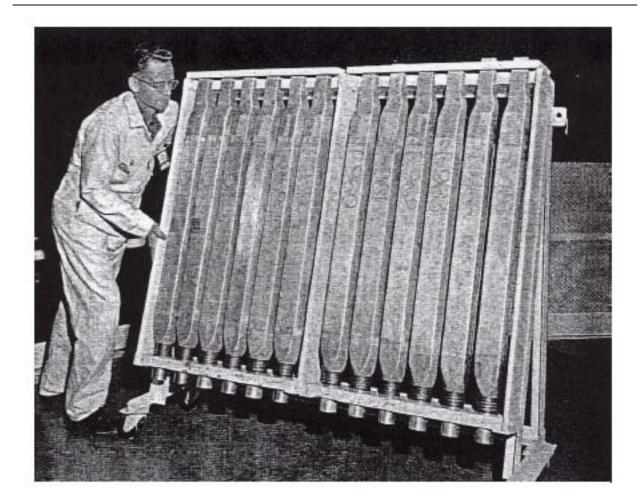
Figure 4-3 Fuel-assembly units
