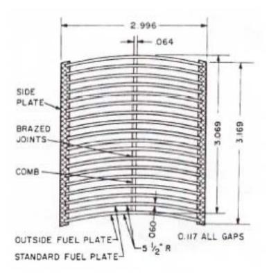
Figure 4-2 Cross section of fuel assembly
