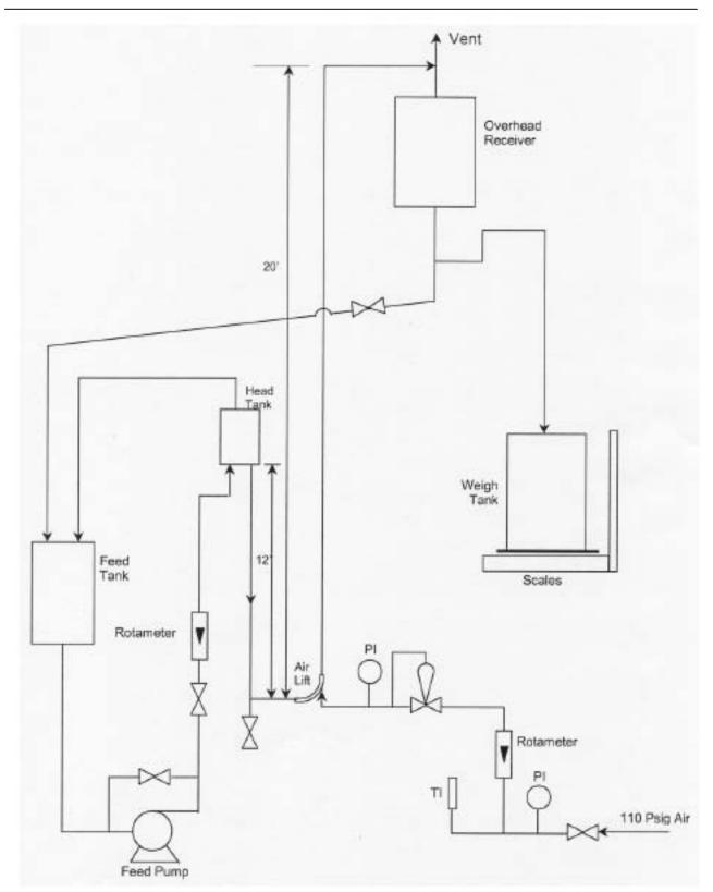
Figure 2-2 Illustration of air-lifting RaLa solutions (Legler et al. 1957)
