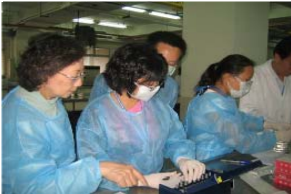
To be able to conduct Salmonella serotyping in their home countries, training participants practice with antisera kits.
