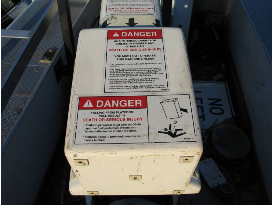
Figure 2 – Vehicle-mounted aerial lift fall hazard danger decal
