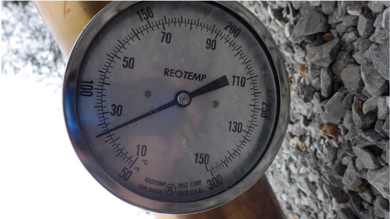
Photo #4: The temperature gauge on the column. (Photo courtesy of the State Fire Marshall)
