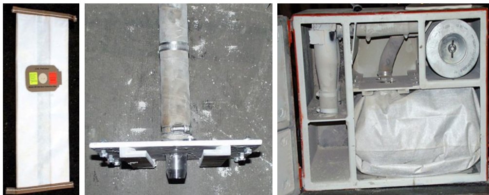
Figure 4.22. Dust collector bag (left), bag nozzle (center), and bag positioned in collector box and filled with dust (right).
