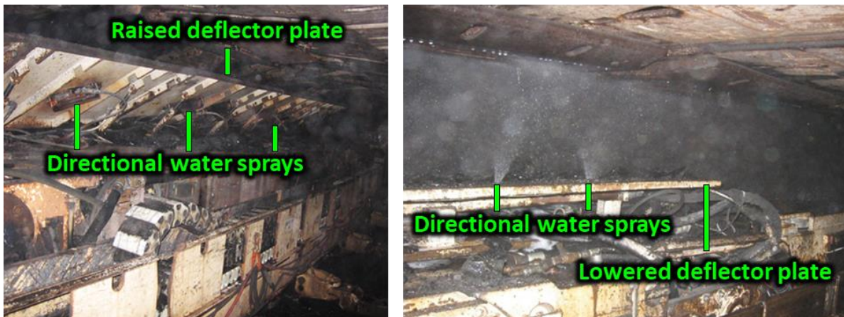
Figure 3.27. The use of deflector plates to enhance the effectiveness of directional water sprays. A raised deflector plate (left) can enhance the effectiveness of the directional spray system by providing a physical barrier and additional directional sprays. When the deflector plates are lowered, sprays can impact the underside of the shields, creating turbulence (right).
