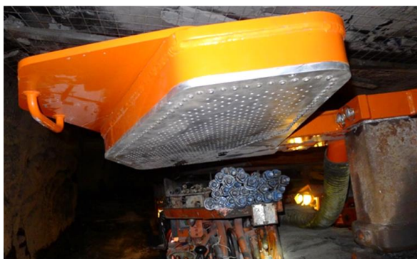
Figure 4.24. Canopy air curtains installed on roof bolters at two underground coal mines.
