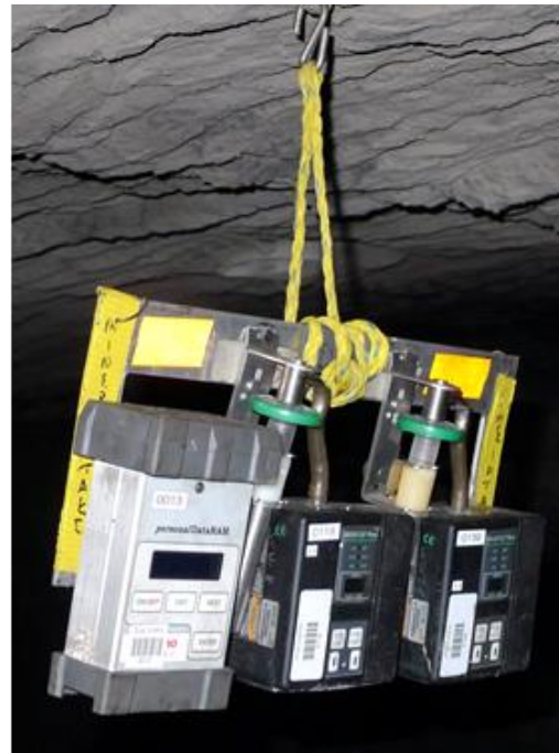
Figure 2.4. pDR 1000AN sampler (left) and pDR operated with gravimetric samplers in an underground coal mine (right).
