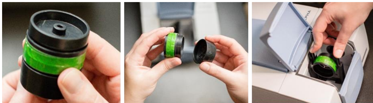
Figure 2.7. Four-piece cassette (left) with filter contained within two center sections (center) and being loaded into an FTIR instrument cradle (right).
