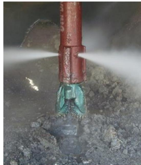
Figure 5.11. Schematic showing internal components of water separator sub (left) and water being discharged through weep holes (right).
