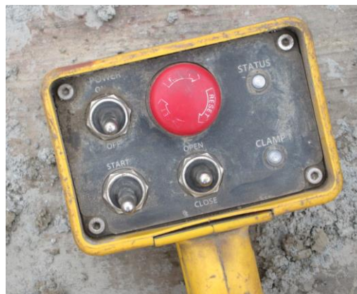
Figures 4 and 5. Vibratory hammer wireless remote control. Below is a drawing with the safety trigger option.
