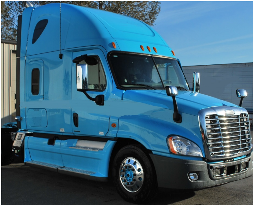
Photo 6: Hood-mounted convex mirrors extend the driver’s field of view along the sides of the truck and trailer.
