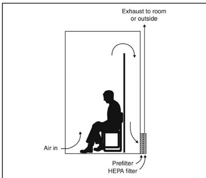
housing and booth is negative compared with adjacent areas. Uncontaminated air from the room will flow into the booth through all openings, preventing infectious droplet nuclei in the booth from escaping into the room. Additional information on the installation, maintenance, and monitoring of HEPA filters is included in this report (Appendix A).
