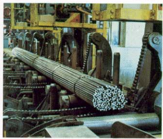
Automatically under computer control, bars are sheared to length, gathered, weighed, and banded into compact, even-end bundles.
