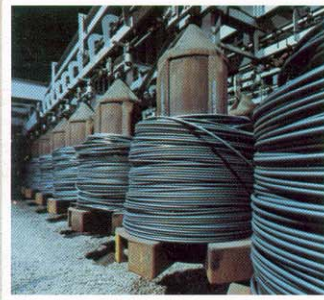
Each coil's identity is continually verified by computer as it moves through the mill on its mandrel.
