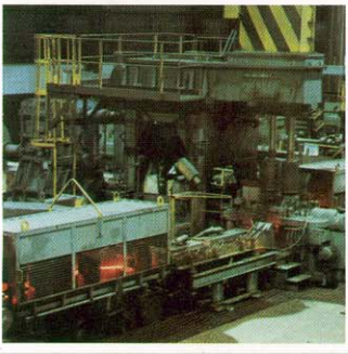
Nine interstand loopers assure tension-free rolling. Computer-controlled water boxes maintain proper bar temperatures.
