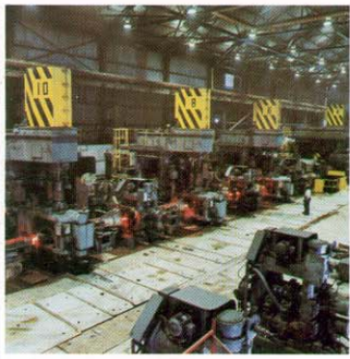
Alternate horizontal and vertical rolls severely work the hot steel as they reduce it in section. This improves the steel's soundness, mechanical properties, and surface.
