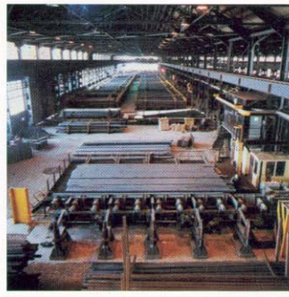
Two charging tables feed billets into furnace after computer verifies billet identity and weight.
