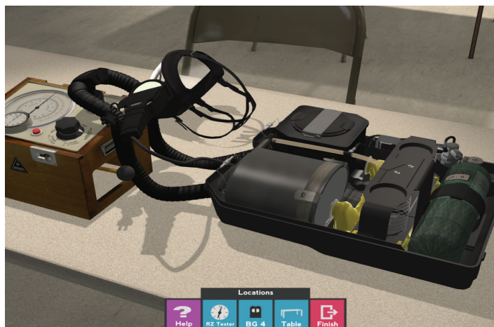
Figure 3: A completely assembled virtual BG 4 attached to the RZ tester unit within the software.
