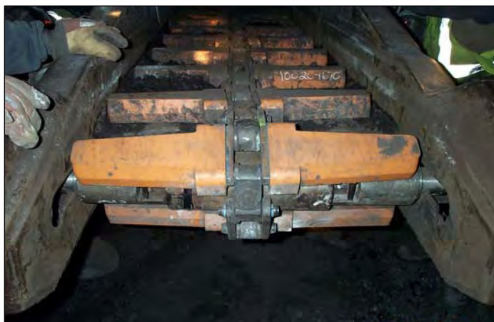
Figure 1.—Urethane-coated flight bar chain.
