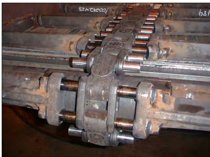
Figure 2.—Dual-sprocket driven chain.
