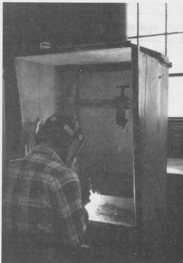
Figure 1. Typical welding operation within the ventilated booth.
