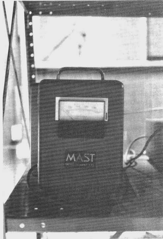
Figure 53. Photograph of the Oxidant Monitor installed for testing.
