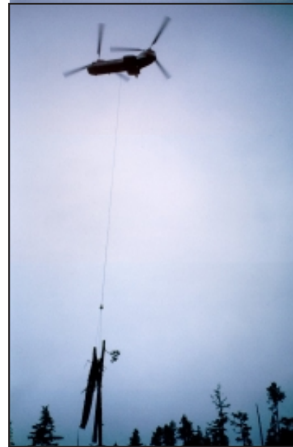
Photo 6: A long line load of logs being lifted by a multi-engine, heavy-lift helicopter
