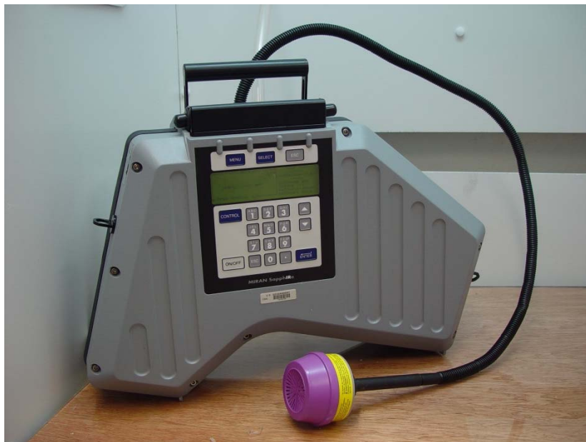
Figure 1. Miran SapphIRe shown with a combination particulate and organic vapor filter cartridge installed on the sampling inlet. The filter cartridge is used for zeroing the instrument prior to test initiation. (Photo Credit: NIOSH)
