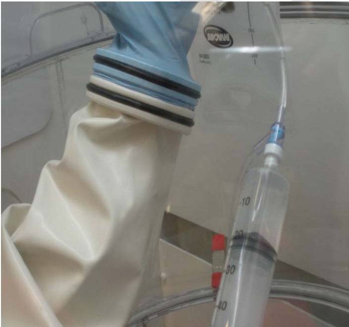
Figure 4b. Photograph showing one of two 60 mL syringes pushing the IPA into the Y-site on an IV administration set (no CSTD shown). (Photo Credit: NIOSH)
