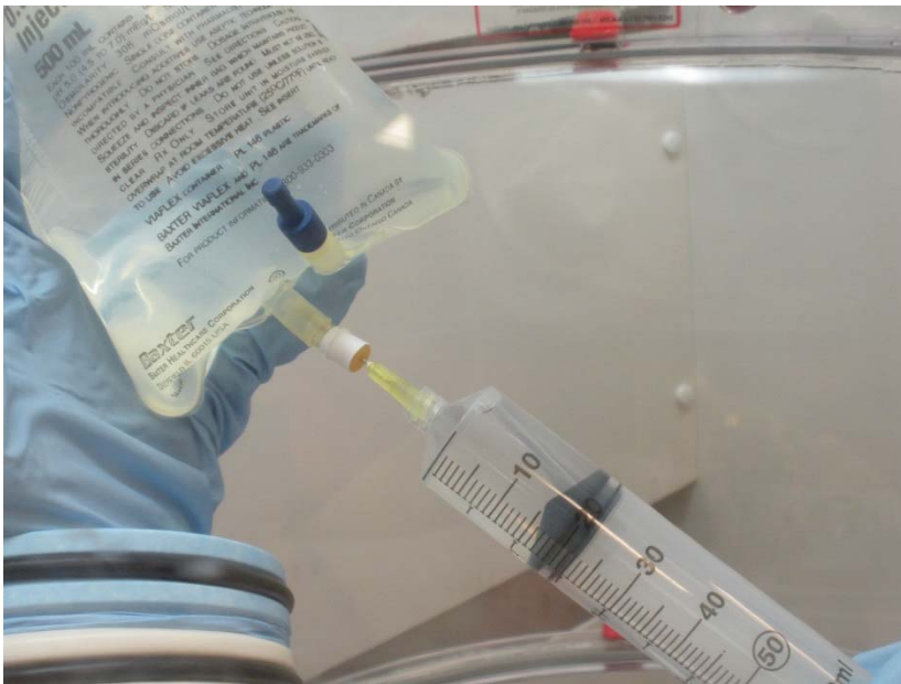
Figure 2. Photograph showing the injection of one of two 45 mL doses of 70% IPA into a 500 mL 0.9% sodium chloride IV bag (no CSTD shown). (Photo Credit: NIOSH)
