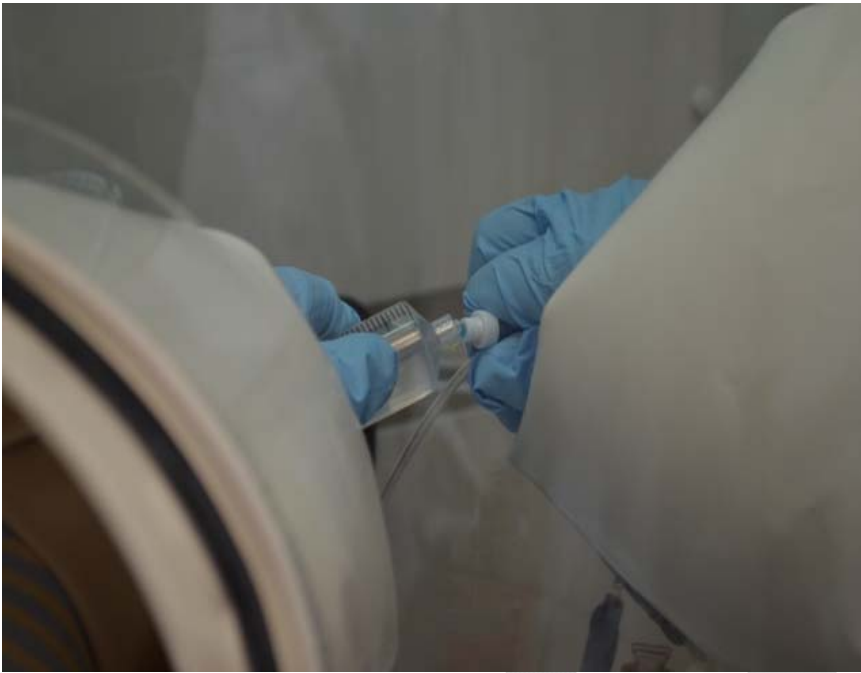
Figure 4a. Photograph showing one of two 60 mL syringes connecting to the Y-site on an IV administration set (no CSTD shown). (Photo Credit: NIOSH)
