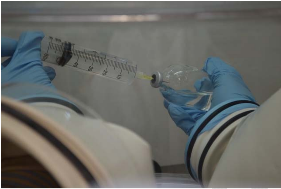
Figure 3. Photograph showing the transfer of 45 mL of 70% IPA from a septum-capped vial into one of two 60 mL syringes (no CSTD shown). (Photo Credit: NIOSH)
