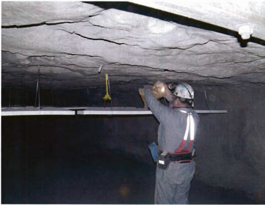
Figure 7. Placing coal and rock dust mixture on shelves in the LLEM.
