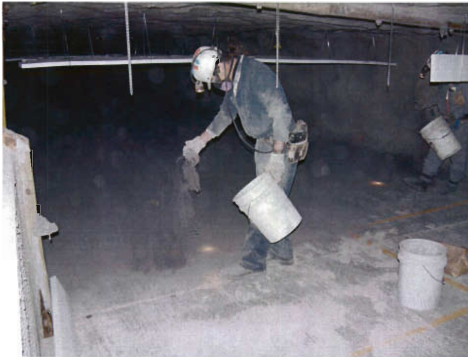
Figure 8. Distributing test dust mixture at the LLEM.
