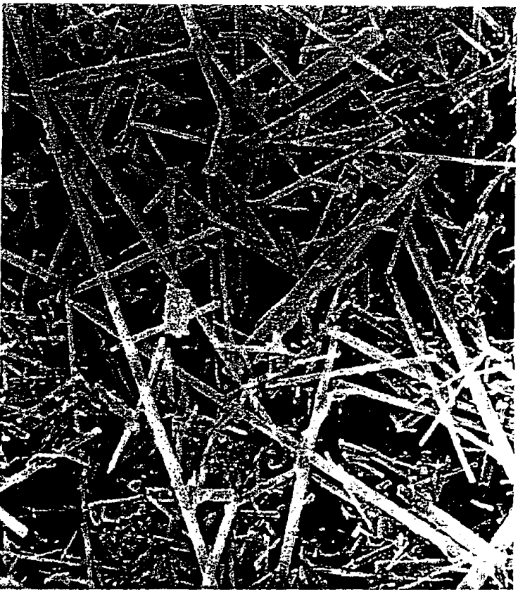
FIGURE 2. Tremolite sample No. 2. Korean tremolite ( \times 10,500 ).
