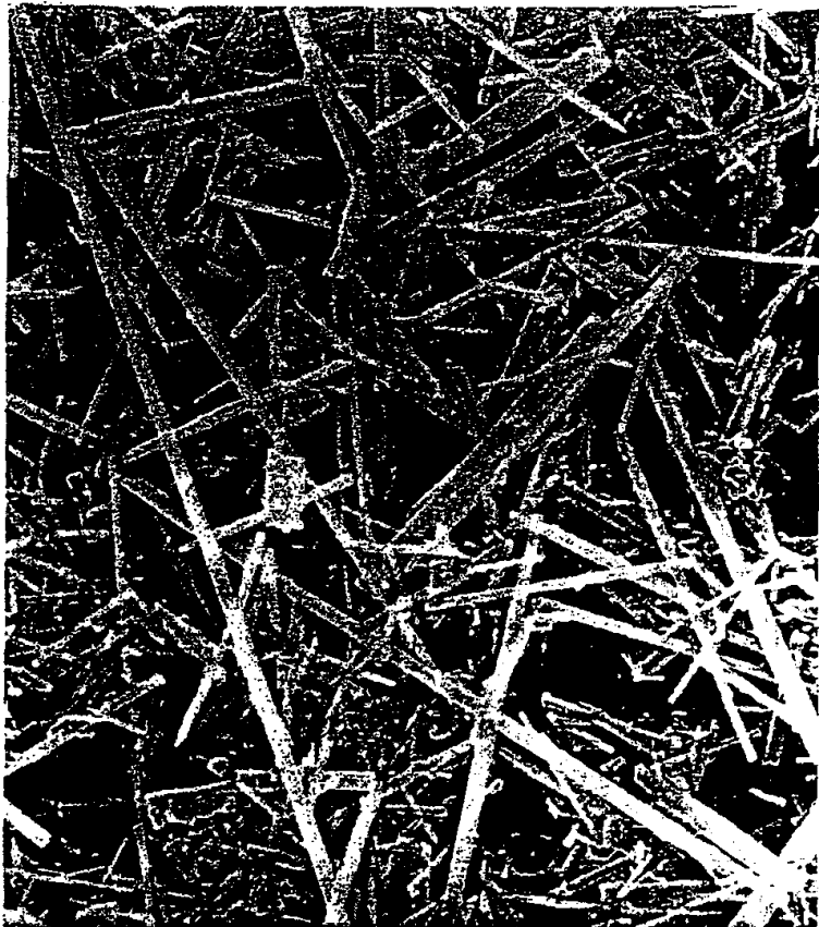
FIGURE 2. Tremolite sample No. 2: Korean tremolite ( \times 10,500 ).
