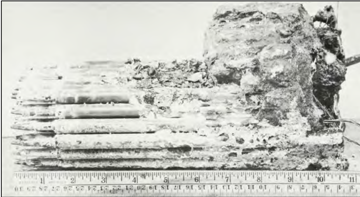
Figure 5-9: View of Melted Mark II Core Assembly
