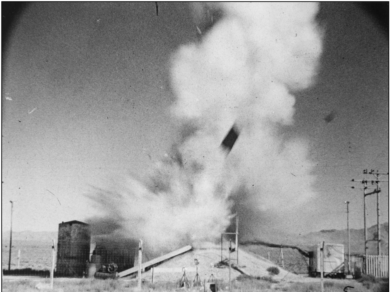
Figure 5-48: Destructive Test of BORAX-I
