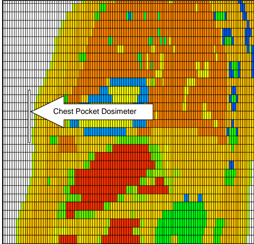
Figure B-6. Elevation view of the adult male voxel phantom showing the left chest pocket dosimeter location.
