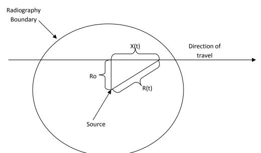
The dose received by an individual walking through a radiography area can be calculated using the diagram provided above. The source is represented by the center of the circle while the circle represents the delineated boundary of the radiography area. The horizontal arrow represents the path taken by the individual through the delineated area. The closest distance the person come to the source is indicated as Ro and the distance from the source at any time t is R(t).
