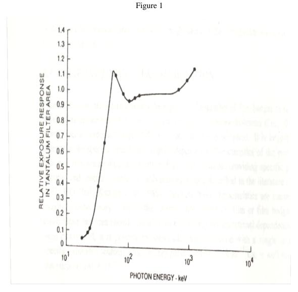
Film response with 0.020 inch tantalum filter (adapted from Brady and Iverson 1968)
