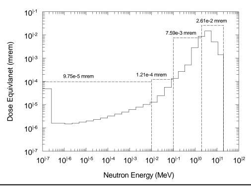
Figure 6-2. Results of neutron spectrum measurements made at 1 m from bare <sup>252</sup>Cf fission neutron source (Soldat and Tanner 1992) (See Y-12 TBD, Fig. 6.3.4.2-3).
