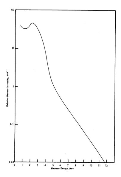
Figure 6-2.ª RTG Plutonium Source Neutron Energy Spectrum – PuO<sub>2</sub> Microspheres. a. (Burkhart, 1987a)
