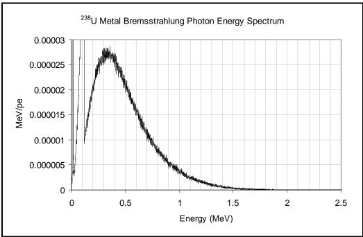
Figure 6-7. *Bremsstrahlung* component of calculated spectrum from <sup>238</sup>U spheres on linear vertical axis. Source: Calculations made using Los Alamos 2003.
