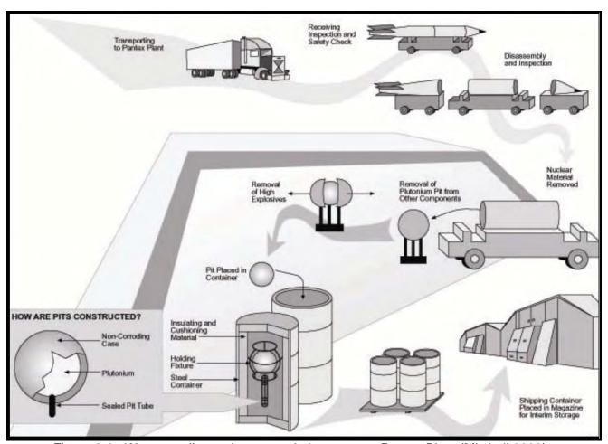
Figure 2-3. Weapons dismantlement and pit storage at Pantex Plant (Mitchell 2003).
