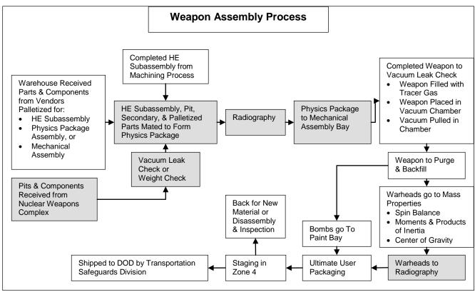
Figure 2-2. Pantex nuclear weapon assembly process (Mitchell 2003).
