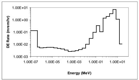
Figure 6-9. Neutron energy spectrum in RASCAL Room 102 at 130 cm from the <sup>238</sup>Pu:Be neutron calibration source.
