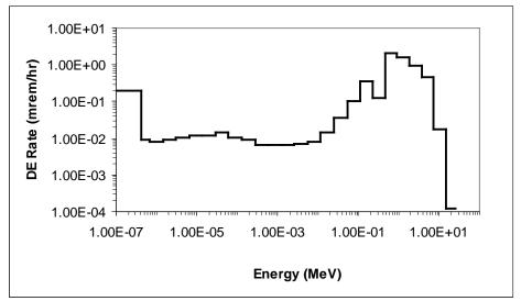
Figure 6-3. Neutron energy spectrum measured by PNL for drums of <sup>241</sup>Am-oxide in Building 3100.
