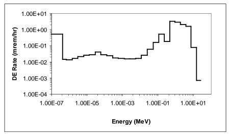
Figure 6-5. Neutron energy spectrum in the RADCAL beta/X-ray irradiation room with a bare <sup>252</sup>Cf source exposed in the adjacent neutron irradiation room.
