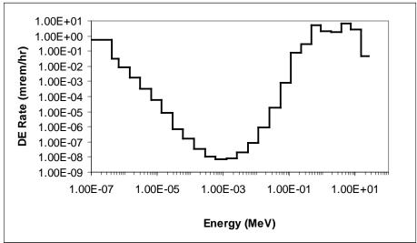
Figure 6-2. Neutron spectrum measured by PNL for <sup>238</sup>Pu:Be and <sup>252</sup>Cf sources in a water-shielded drum in Building 3038.
