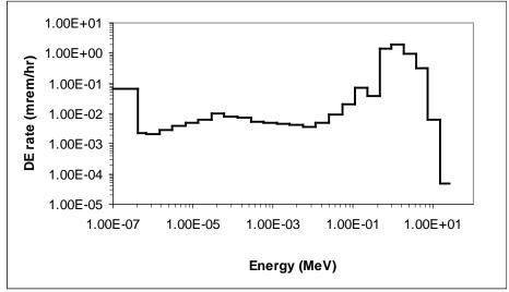
Figure 6-10. Neutron energy spectrum measured by PNL in REDC Room 111 at 37 cm from a glovebox containing <sup>252</sup>Cf.
