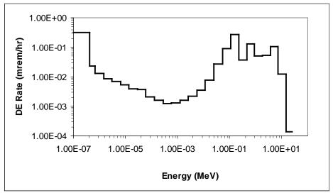
Figure 6-7. Neutron energy spectrum in the hallway outside the RADCAL neutron irradiation room with a moderated <sup>252</sup>Cf source exposed.
