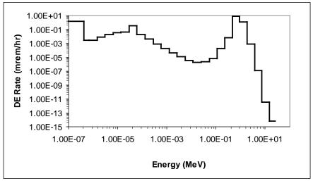
Figure 6-6. Neutron energy spectrum in the RADCAL beta/X-ray irradiation room with a moderated <sup>252</sup>Cf source exposed in the adjacent neutron irradiation room.
