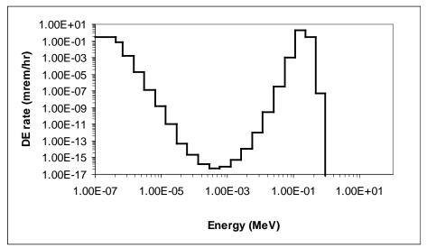
Figure 6-12. Neutron energy spectrum for the REDC TDF containing 12 mg <sup>252</sup>Cf.
