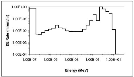
Figure 6-8. Neutron energy spectrum in the RADCAL equipment room with a moderated <sup>252</sup>Cf source exposed in the adjacent neutron irradiation room.
