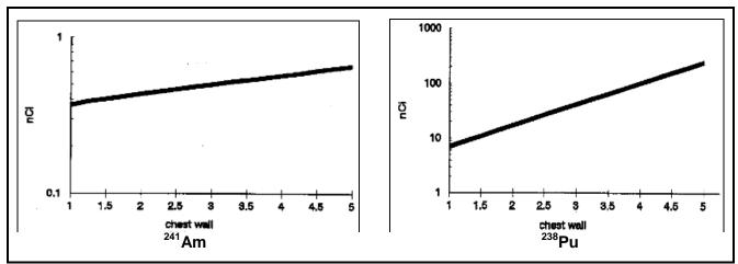
Figure 5-2. Current MDA values (nCi) for ORNL phoswich lung counter versus chest-wall thickness (cm) for <sup>241</sup>Am and <sup>238</sup>Pu (Watts et al. 1995).
