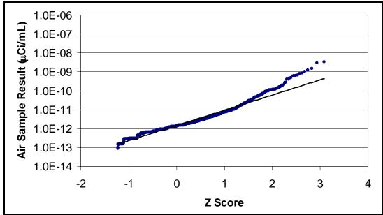
Figure 5B-4. Alpha air-monitoring results for 1944-1947. The geometric mean =  $1.4 \times 10^{-12} \,\mu\text{Ci/mL}$ , the GSD = 6.35, and  $r^2 = 0.97$ .
