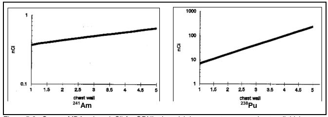
Figure 5-2. Current MDA values (nCi) for ORNL phoswich lung counter versus chest-wall thickness (cm) for <sup>241</sup>Am and <sup>238</sup>Pu (Watts et al. 1995).
