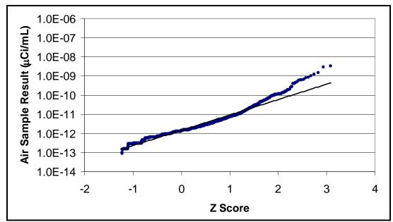
Figure B-4. Alpha air-monitoring results for 1944–1947. The geometric mean =  $1.4 \times 10^{-12} \,\mu\text{Ci/mL}$ , the GSD = 6.35, and  $r^2 = 0.97$ .
