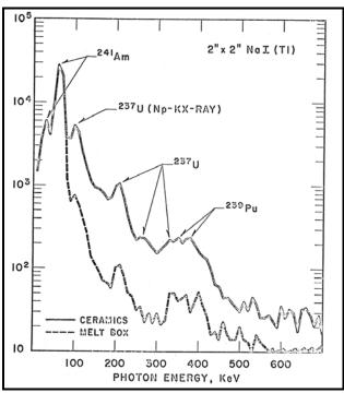
Figure 6-2. Gamma spectrum external to plutonium ceramics line and plutonium melt glovebox (Caldwell and Judd 1966, Figure 4).
