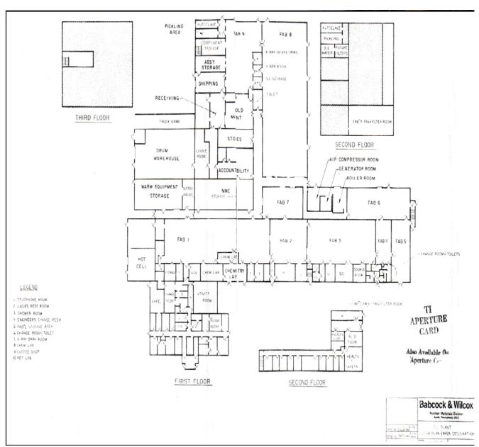
Figure 2-6. Parks Township Plutonium Plant (Building A) layout (Austin 1979).
