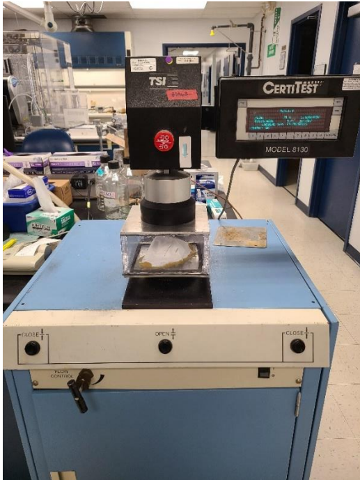
Figure 2: Laboratory Test Photo (TSI, Inc. 8130 filter tester)
