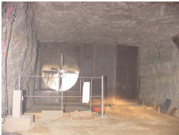
Figure 6. Large propeller fan mounted in bulkhead
