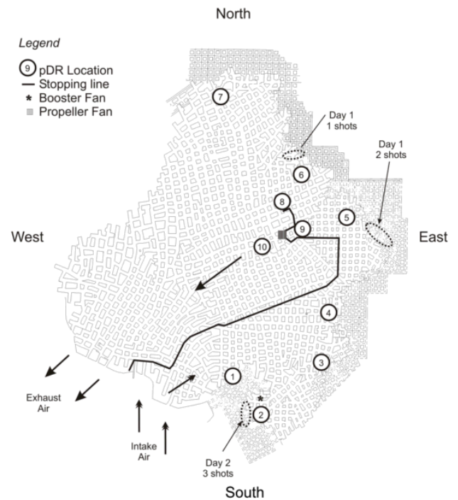
Figure 6 - Mine workings for case study, showing location of dust monitors, curtain line, and fans.
