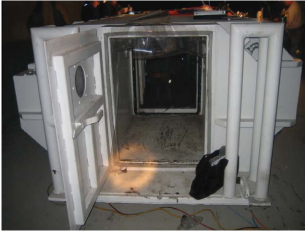
Fig. 1. Photograph of the entrance to a refuge chamber.
