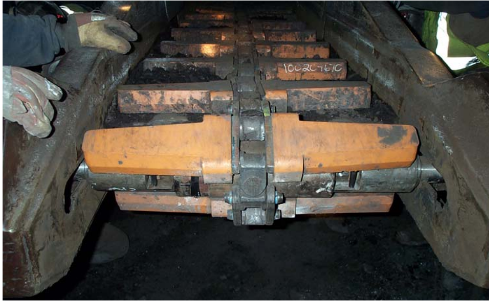
Figure 2: Coated conveyor flight bars on a continuous mining machine.
