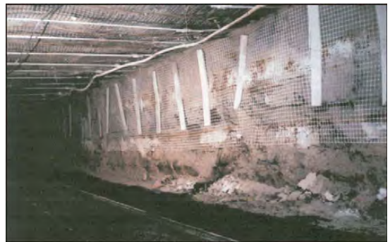
Figure 4 Synthetic mesh supporting roof and rib. (Photo courtesy of Tensar Earth), (Bauer and Dolinar, 2000).
