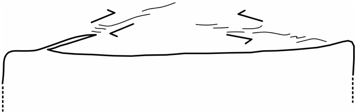
Figure 1.—Representative cross section showing fracture patterns in halite roof. (Modified from [6]: Figure 6.)
