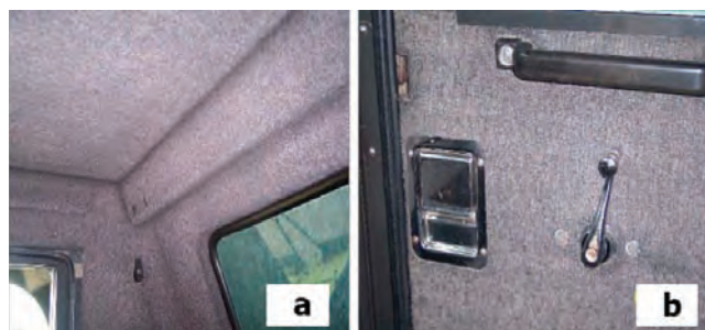
Examples of new-style cab, a) full-upholstery and window seals b) newer gaskets, door handles and window cranks.
